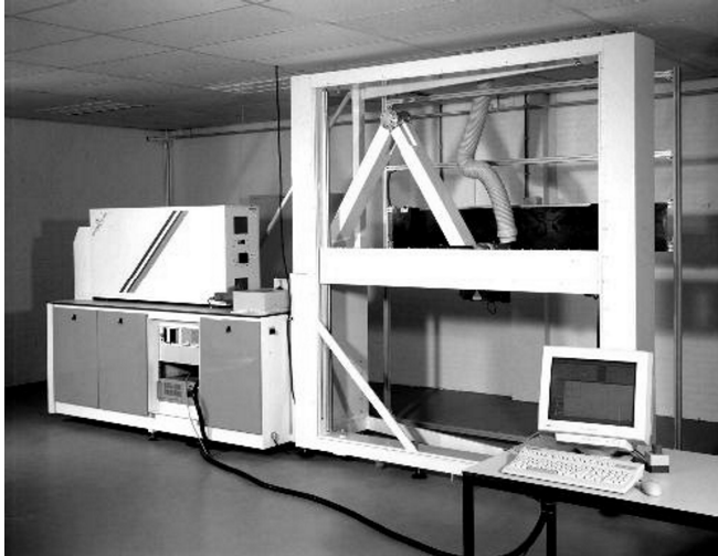
Fig. 2.3 Photograph of the “Advanced workstation for controlled laser cleaning of artworks” [source: Art Innovation]
