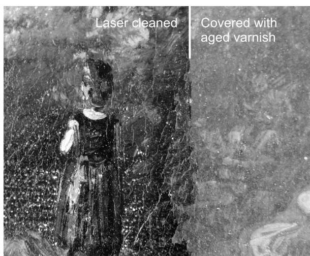
Fig. 2.5 Fraction of an oil painting with aged varnish layer. The left side is laser cleaned with a KrF-excimer laser [source: J. Hildenhagen, LFM]
