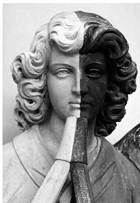
Fig. 2.4 Angel figure of the Cologne cathedral (Germany). The left half is laser cleaned with a Nd:YAG laser. The right half is untreated [source: Bauhütte Naumburg]
