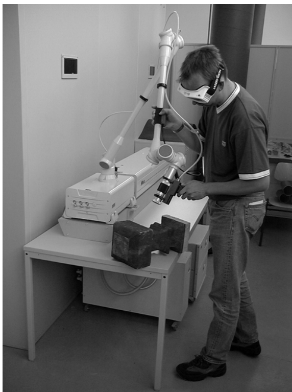
Fig. 3.4 Removal of an encrustation layer on sandstone with the Nd:YAG cleaning laser
